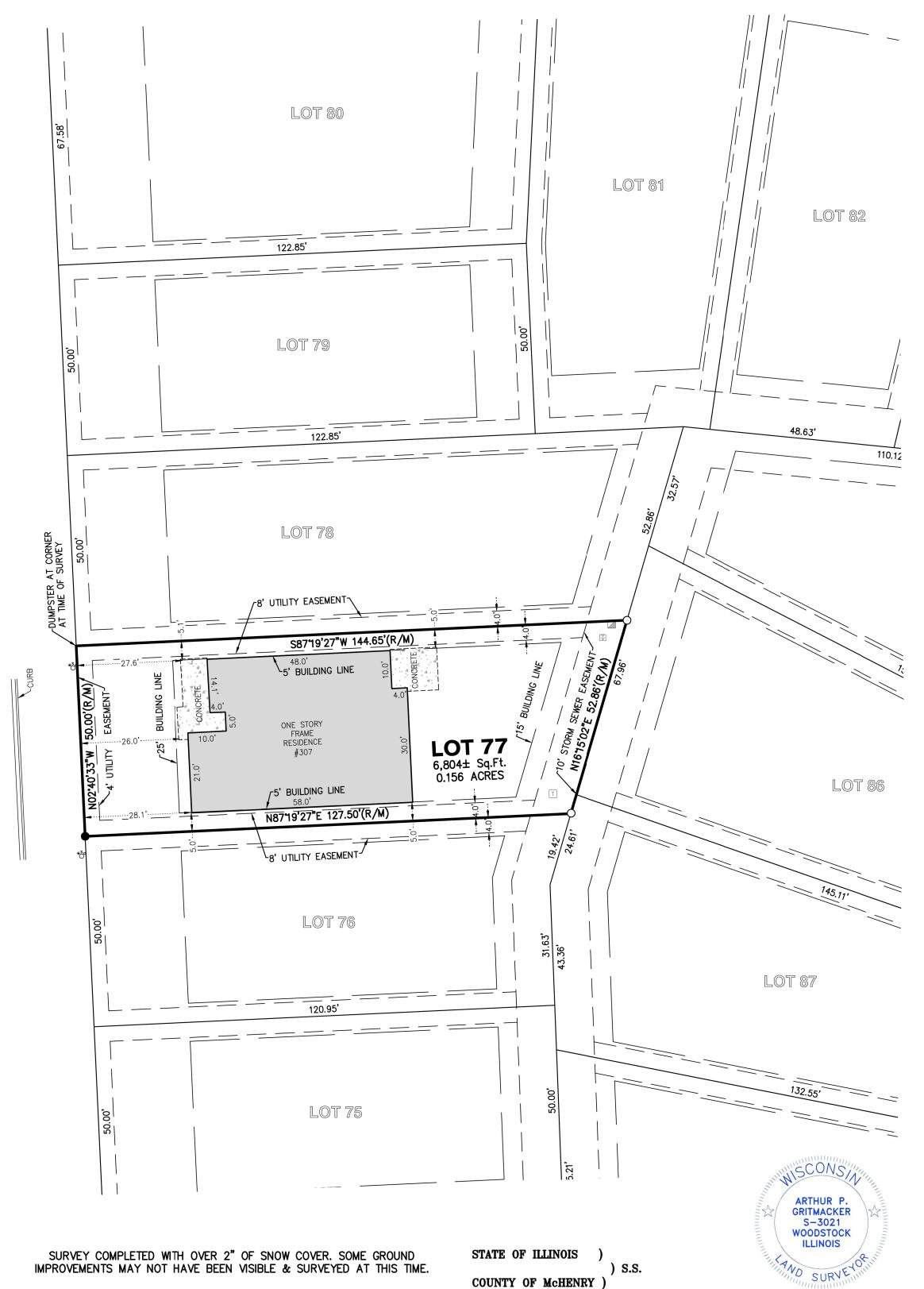
**LEGEND** ELECTRIC RISER FOUND IRON BAR 0 FOUND IRON PIPE  $\otimes$ FOUND MAG NAIL  $\boxtimes$ FOUND MONUMENT ₩ SET CROSS SET IRON BAR ⊗ SET MAG NAIL T TELEPHONE RISER  $\overline{\Psi}$ TV RISER
